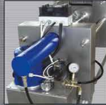
Otomatik, Hidrolik Kapatma Sistemi. Automatic, hydraulic closure system.
